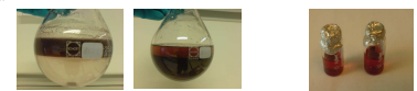
Figure 8: Left and middle: AuNPEG extracted from water to methylene chloride. Right two AuNPEG samples after overnight sterilization cycle in autoclave
